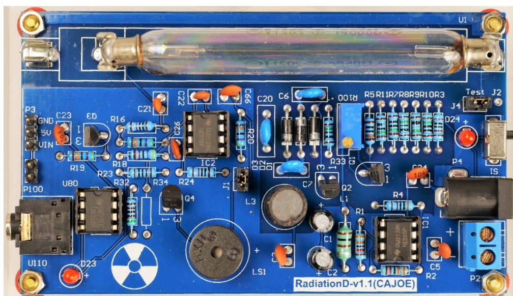
Obr. 4.4: GM detektor RadiationD-v1.1(CAJOE) s trubicou J305β.
