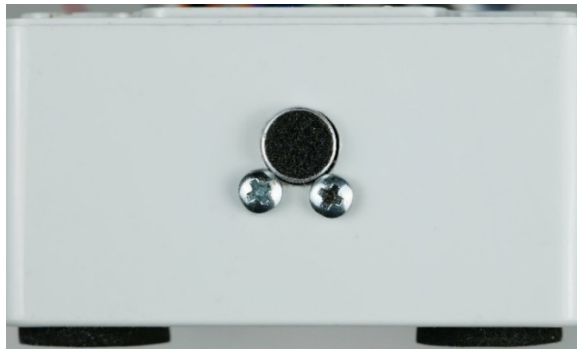
Figure 3.12. Mounting the microphone sensor
