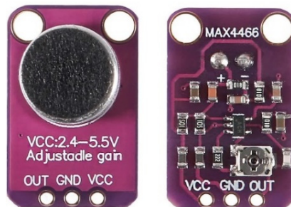
Figure 3.4. Electret microphone with operational amplifier MAX4466
