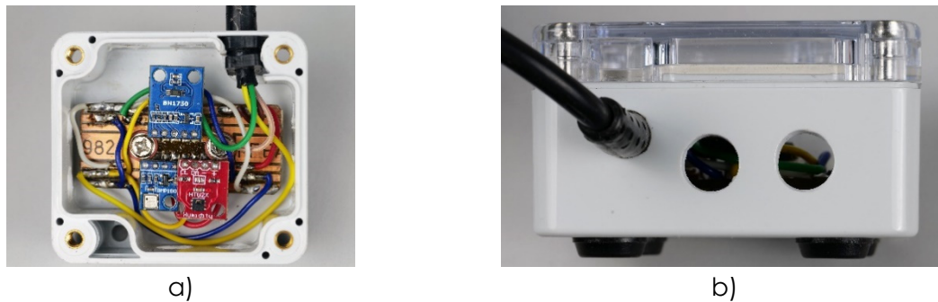
Figure 5.9a, b. Mounting the sensors on the printed circuit board and fixing the printed circuit board with the sensors in the assembly box with a transparent top cover (a), view of the drilled holes from the side of the box (b)
