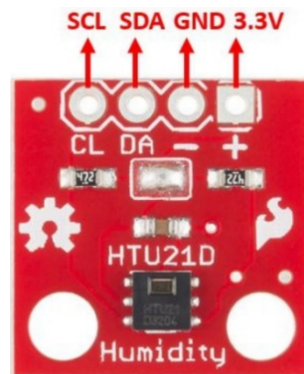
Figure 5.6. HTU21D sensor designed for measuring relative humidity and air temperature
