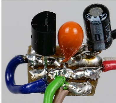
Figure 3.6. Voltage stabilizer LP2950ACZ-3.3/NOPB with 1 \mu\text{F} and 2.2 \mu\text{F} capacitors, located on the PCB and powered by the 5 V DC output of the Arduino
