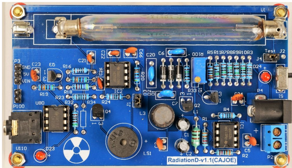
Figure 4.4. RadiationD-v1.1(CAJOE) GM detector with J305β tube
