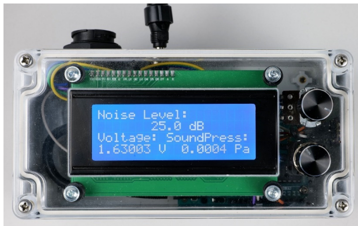
Figure 3.1. Sound meter with Arduino Uno microcontroller
