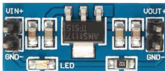
Figure 3.5. AMS1117 3.3V voltage stabilizer, powered by 5V DC output of Arduino
