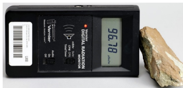
Figure 4.8. Measurement of uraninite activity using GM detector Vernier TH30044
