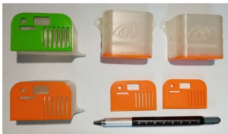
Figure 7.4. Covers and protective boxes for environmental sensors – you can see the scale (using the pen next to the two orange covers). They were made from PLA.
